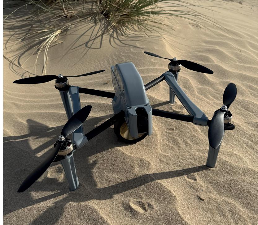
FPV – UAV 9" for attack or intelligence missions. It can be used in navigation modes and fly on assignment. Uses LORA, ELRS, CRSF protocol control. The ability to install up to 3 receivers with packet separation in case of loss of communication.
