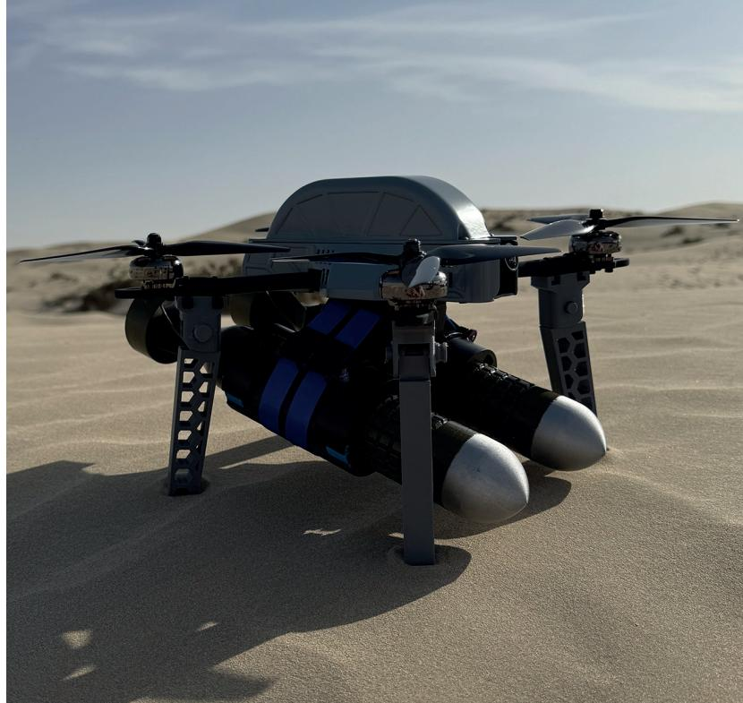
FPV – UAV 7" for attack or intelligence. It can be used in navigation modes and fly on assignment. Uses LORA, ELRS, CRSF protocol control. The ability to install up to 3 receivers with packet separation in case of loss of communication.
