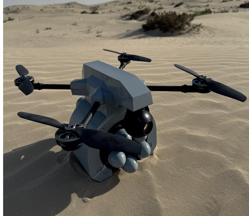
FPV – UAV 13" for attack or intelligence missions. It can be used in navigation modes and fly on assignment. LORA, ELRS, CRSF protocol control. The ability to install up to 3 receivers with packet separation in case of loss of communication.
