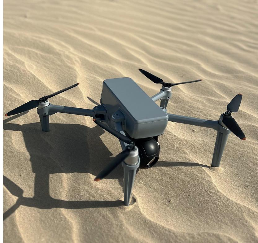
Attack UAV with the function of dropping striking elements. It can be used in navigation modes and fly on assignment. Uses LORA protocol control. The ability to install up to 3 receivers with packet separation in case of loss of communication.
