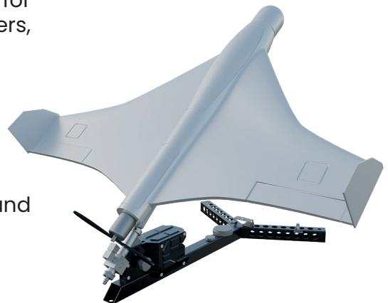
The primary structure, or airframe, crafted from lightweight composite materials, provides the essential aerodynamic design that allows for high endurance and stability during long missions.
